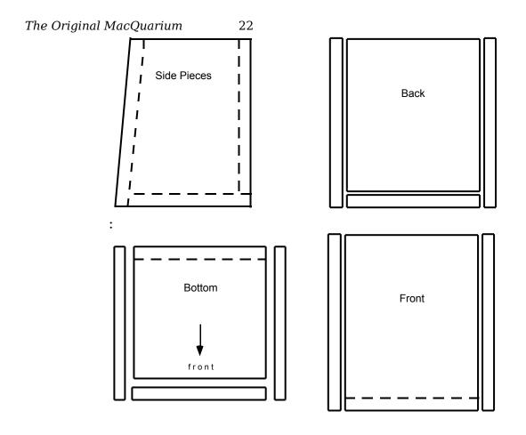
From the guide, you can see that the side panels are supposed to go on top of everything else, while the back panel is surrounded by glass on all four sides.
